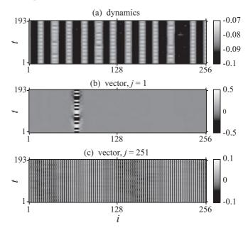
FIG. 21. Spatiotemporal evolution of the dynamics  $x_i^t$  (a), of a physical Lyapunov mode at j = 1 (b), and of a spurious Lyapunov mode at j = 251 (c) in the coupled tent maps with K = 0.65. The spatial profiles are plotted every eight time steps in order to capture the internal structure of the period-4 collective behavior.
