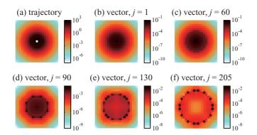
FIG. 29. (Color online) Power spectrum  $S(k_x, k_y)$  of the trajectory (a) and of the CLVs (b)–(f) for the 2D KS equation. The spectra are shown for  $k_x, k_y \in [-k_{cut}, k_{cut}]$  with  $k_{cut} = 10 \times 2\pi/L$ .
