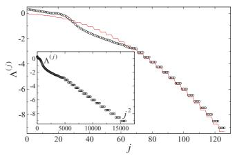
FIG. 9. (Color online) Lyapunov spectrum for the CGL amplitude turbulence. The stepwise structure starts at j = 71. The red dashed line indicates  $\Lambda^{(j)} = 1 - k^2 - 2\langle |W|^2 \rangle$  derived by Garnier and Wójcik for pure Fourier perturbations [36]. (Inset) The same data against  $j^2$ . The Kaplan-Yorke dimension in this case is about 28.6.
