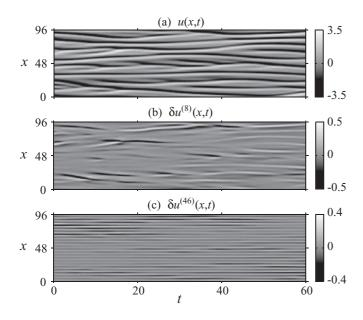
FIG. 2. Typical spatiotemporal structure of the trajectory u(x,t)(a) and CLVs  $\delta u^{(j)}(x,t)$  (b), (c) in the physical and the spurious regions, respectively, for the 1D KS equation (L = 96,  $k_{cut} = 42 \times 2\pi/L$ , PBC). The index of the CLV shown here is j = 8 (b) and j = 46 (c).
