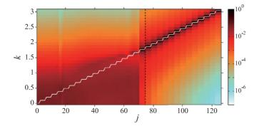
FIG. 11. (Color online) Spatial power spectrum  $S_j(k)$  of the CLVs for the CGL amplitude turbulence, shown as a function of the wave number *k* and the Lyapunov index *j*. Given that  $S_j(k)$  and  $S_j(-k)$  are statistically equivalent, their average is shown in the figure. The black dashed line separates the physical and spurious regions at  $N_{\rm ph} = 74$ . The white solid line indicates  $k = [(j + 1)/4]2\pi/L$ .
